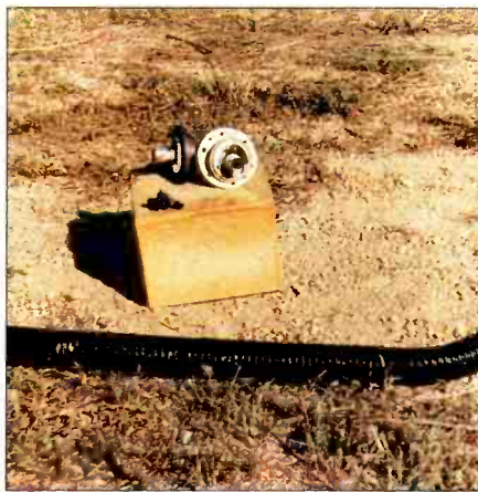
This broadcast line was struck by lightning. The coax was destroyed — even the outside plastic jacket of the coax was melted. The black, charred piece next to the elbow is a melted bullet.
